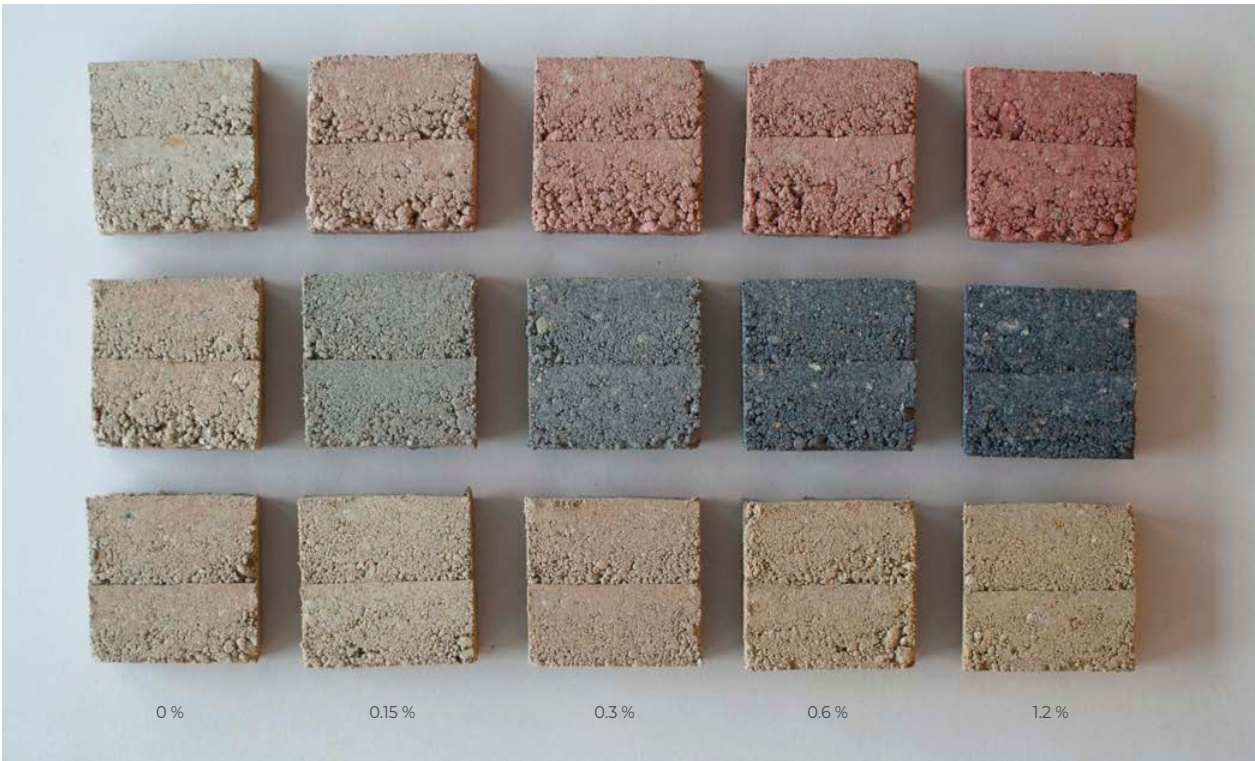
Figure 53. Samples with different quantities of pigmentation.
