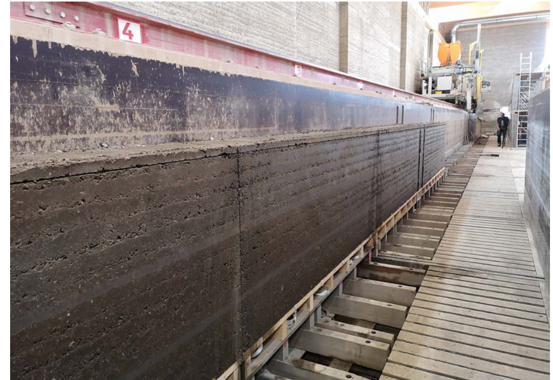
Figure 66. Fresh sliced rammed earth elements. Erden Werkhalle, Schlins.
