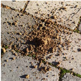
Figure 28. The ball disintegrated in many small pieces.
