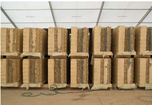
Figure 11. Prefabricated wall elements drying for 4 - 6 weeks.
