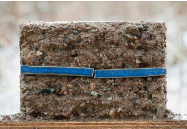
Figure 50. The erosion checks are now fully revealed.
