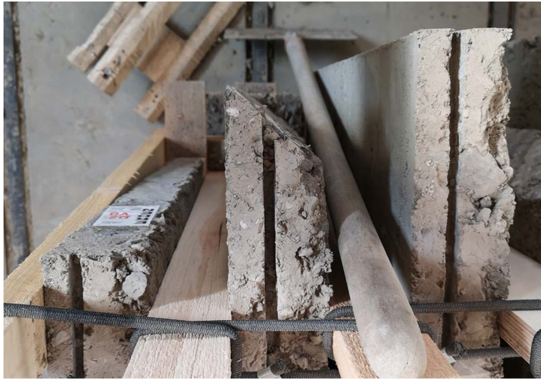
Figure 69. A rammed earth element cut at a 45-degree angle. Erden Werkhalle, Schlins.
