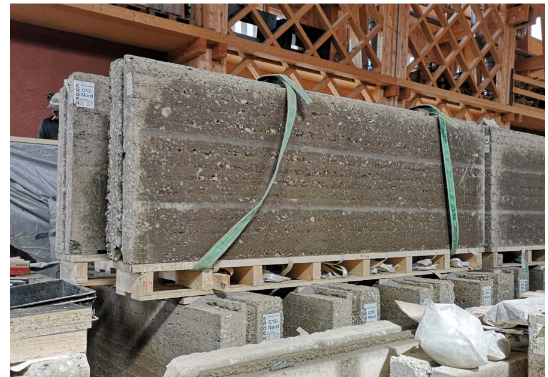
Figure 67. The rammed earth element is starting to dry. Erden Werkhalle, Schlins.
