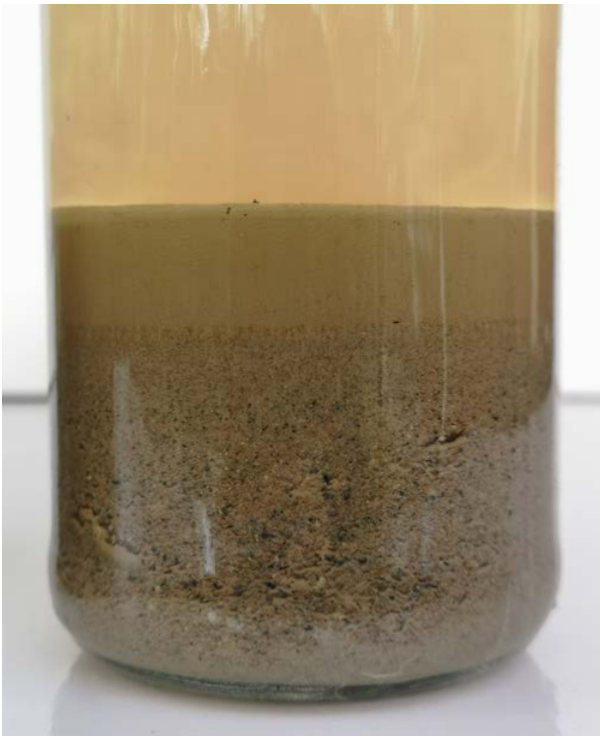
Figure 33. Sediment test of the excavated earth.
