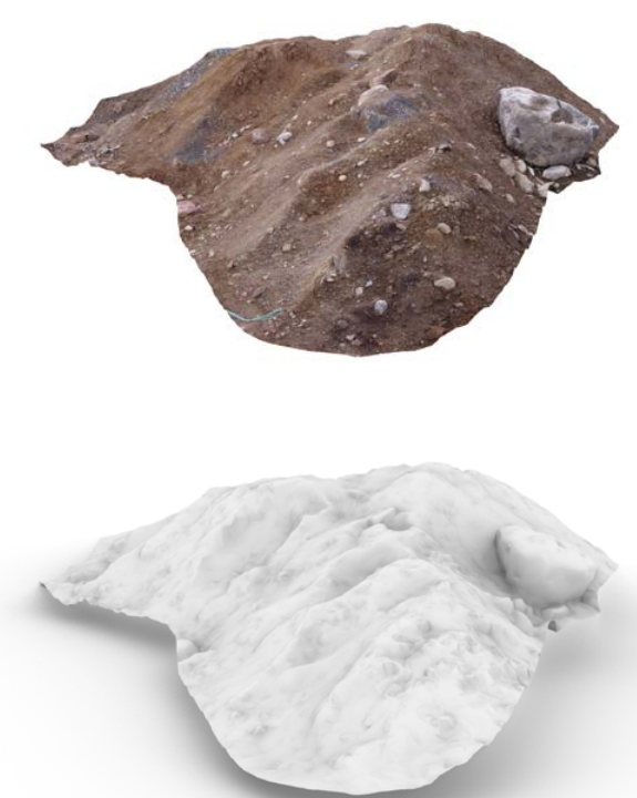
Figure 25. 3D model of the excavated earth pile, obtained from drone photographs and photogrammetry.
