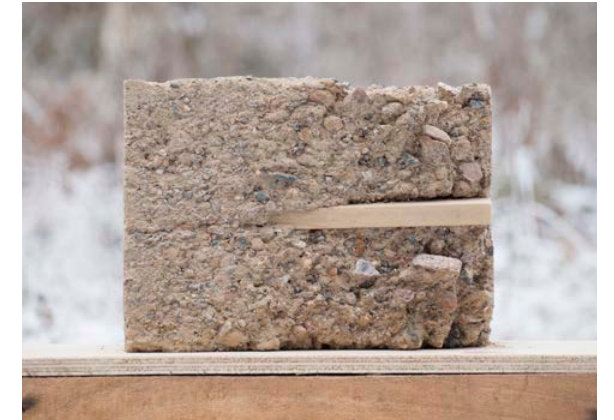
Figure 2. One of the many erosion experiments on rammed earth I conducted during the material exploration.
