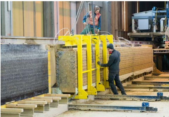
Figure 10. Slicing of the long rammed earth wall into smaller elements.
