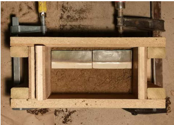
Figure 43. Insertion of ceramic erosion checks.
