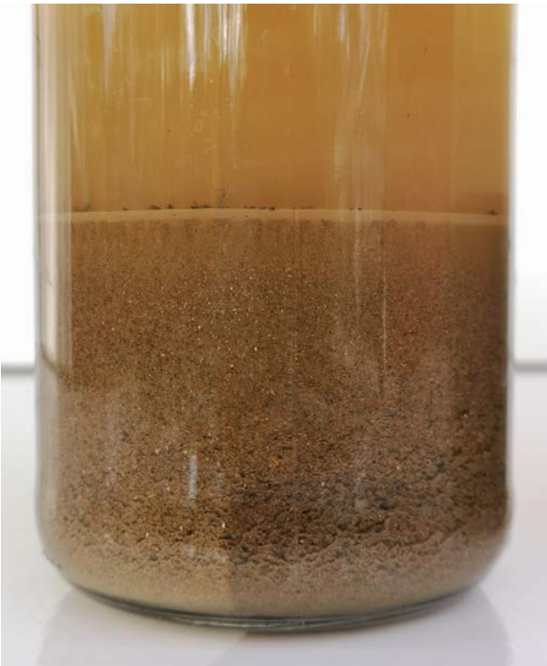
Figure 29. Sediment test of the earth from my parents' garden.
