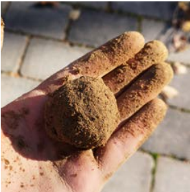
Figure 27. Ball drop test 1.
