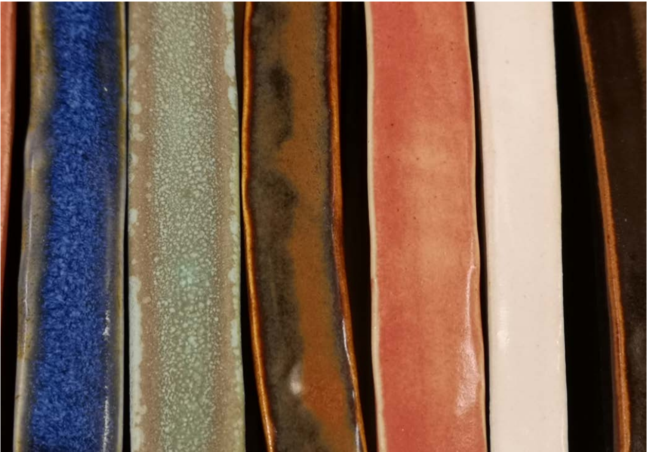
Figure 42. The glazed ceramic tiles with different colours will be used as erosion checks in the rammed earth.
